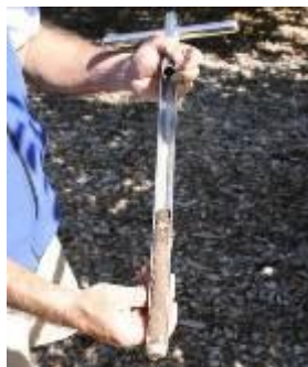
Core of soil for testing.
